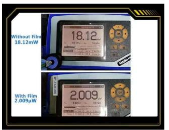
PhotonSafe Laser welding protection
