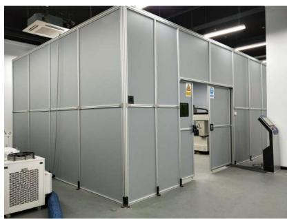
The best way to safeguard a laser environment according to EN 60825-1 and OStrV is to enclosure the whole laser area. Especially in the field of laser material processing with laser powers up to the kW range, this is a very common way to proceed. The cabin will then be designed in a way, that the laser area is still accessible.
